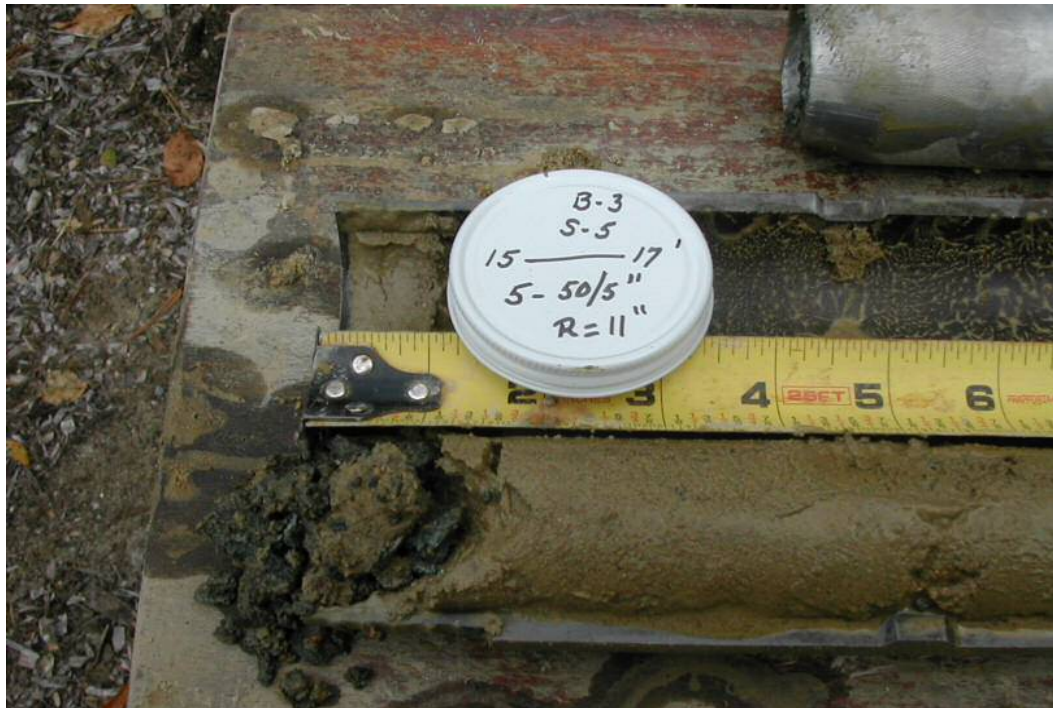
Photo 18: Test boring B-3, S-5: Stratified Sand w/Thin Silt Layers, with Rock Fragments in the tip of the sampler.
