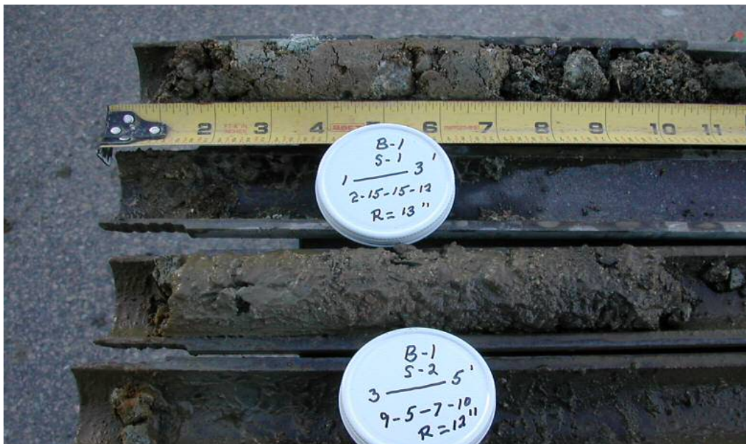
Photo 2: Test boring B-1 split-barrel soil samples S-1 & S-2 from 1.0 to 3.0 ft & 3.0 to 5.0 ft below the existing grade, respectively. For all photographs, the soil samples increase in depth from right to left within the split-barrel sampler. The number of hammer blows to advance the split-barrel sampler in 6-inch increments is shown just below the sampling depth on the sample jar lids. "R" represents the soil sample recovered in inches. Recovered in S-1 & S-2 was Silty Sandy Gravel, saturated at 2.75 ft.
