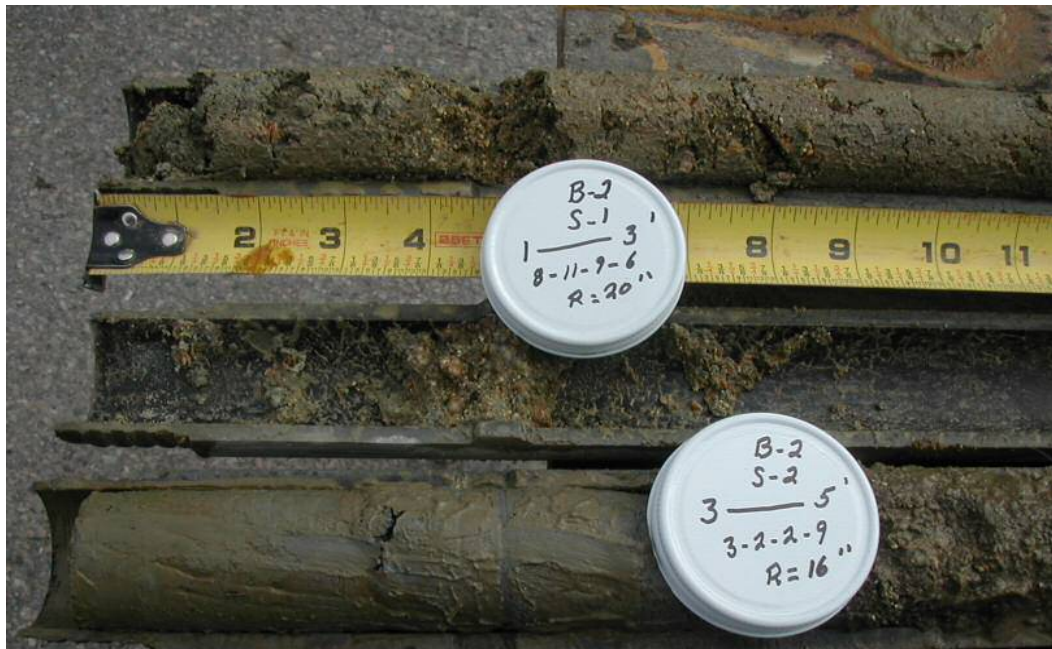
Photo 9: Test boring B-2 split-barrel soil samples S-1 & S-2 from 1.0 to 3.0 ft & 3.0 to 5.0 ft below the existing grade, respectively. Silty Gravelly Sand, c-f Sand, 25-35% subrounded to angular m-f Gravel, 5-15% nonplastic Fines, moist to saturated at 2.5', brown over gray Silt at 4.5 ft, consisting of slightly plastic Fines, 2" brown over gray.
