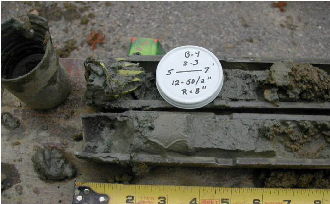
Photo 21: Test boring B-4, S-3: Weathered Rock with Rock fragments in tip of sampler.
