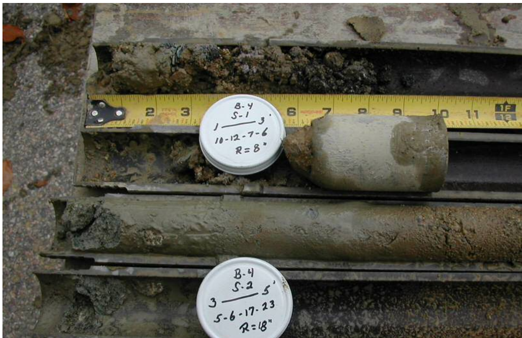
Photo 20: Test boring B-4 split-barrel soil samples S-1 & S-2 from 1.0 to 3.0 ft & 3.0 to 5.0 ft below the existing grade, respectively. Recovered was Silty Gravelly Sand, c-f Sand, 25-35% subrounded to angular m-f Gravel, 5-15% nonplastic Fines, moist to saturated at 2.75' with rock in tip of S-1 sampler. Gray Till transitions to Weathered Rock from 4 to 5 ft.
