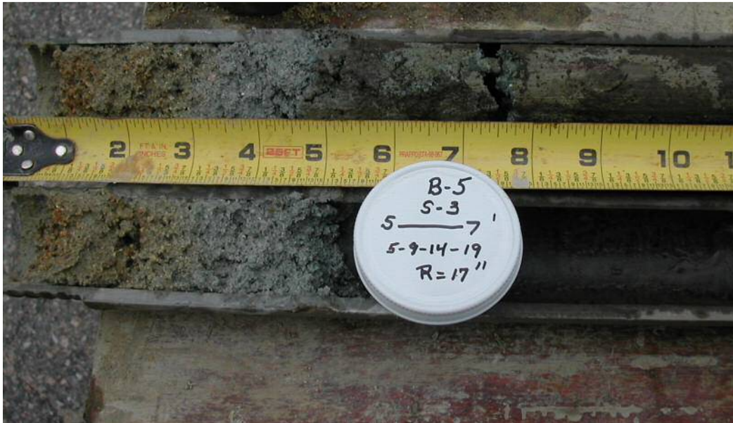
Photo 24: Test boring B-5, S-3: Clayey Silt, slight plastic Fines, saturated, gray transitioning to Silty Sand around 6.5 ft.
