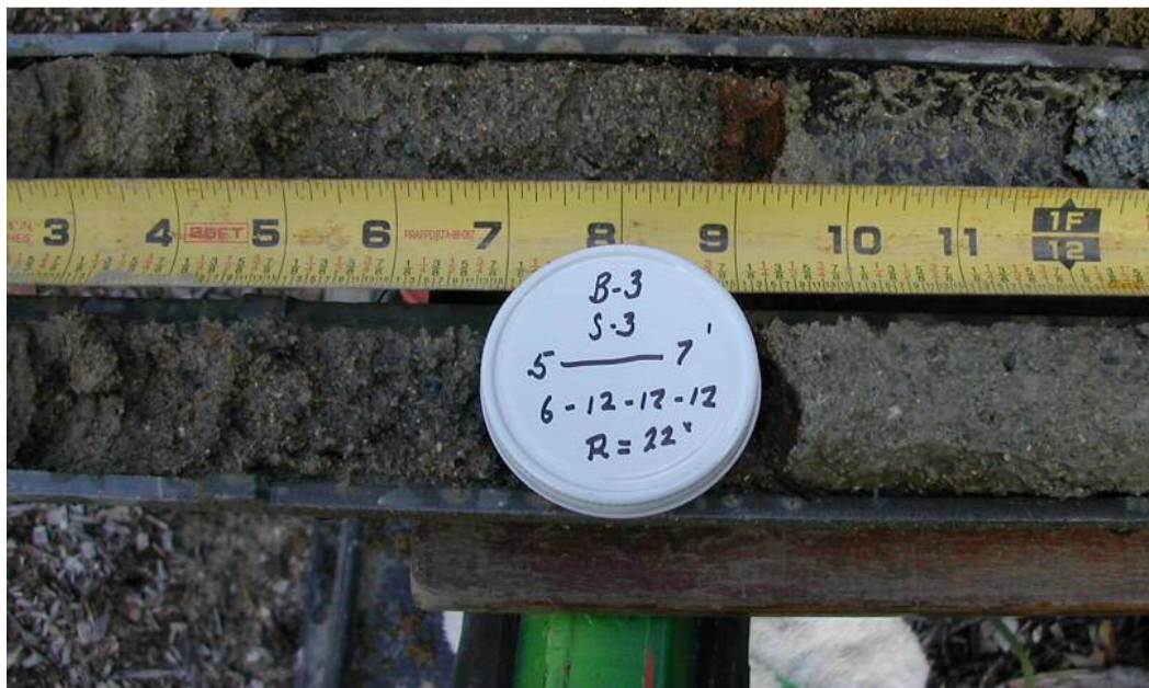
Photo 16: Test boring B-3, S-3: Silty Sand, m-f Sand, 15-25% nonplastic Fines, <5% fine Gravel, gray to brown @ 6'±.
