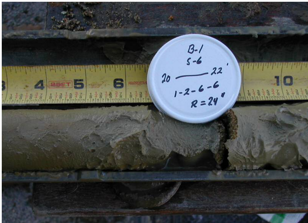
Photo 6: Test boring location B-1, S-6: Silt, nonplastic Fines, 1/16" seam medium, Sand, saturated, grayish brown.
