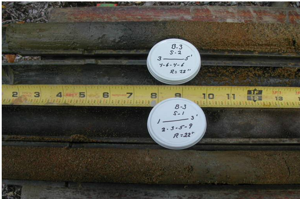
Photo 15: Test boring B-3 split-barrel soil samples S-1 & S-2 from 1.0 to 3.0 ft & 3.0 to 5.0 ft below the existing grade, respectively. Woodchips, Organic Silt and Sand over Organic Silt, blackish to dark gray between 4 and 5 ft, slightly plastic Fines.
