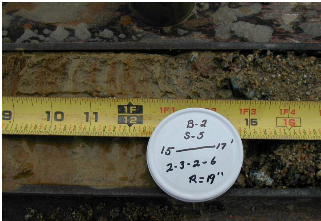
Photo 12: Test boring B-2, S-5 consisted of 6" Gravelly Sand, c-f Sand, 15-25% angular Gravel, <2% nonplastic Fines, brown over stratified fine Sand, with horizontal grayish and rusty brown mottling.
