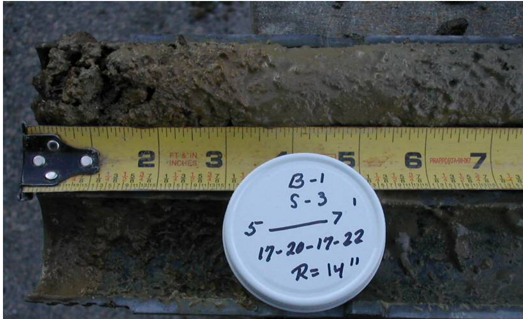
Photo 3: Test boring location B-1, S-3: Silty Sandy Gravel, subrounded to angular m-f Gravel, 30-40% c-f Sand, 15-20% slightly plastic Fines.
