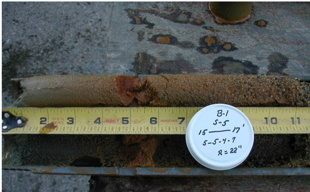
Photo 5: Test boring location B-1, S-5: Sand, stratified, mostly m-f Sand, 2" c-f seam, <5% nonplastic Fines, saturated, dark orange brown – tip gray Silt.
