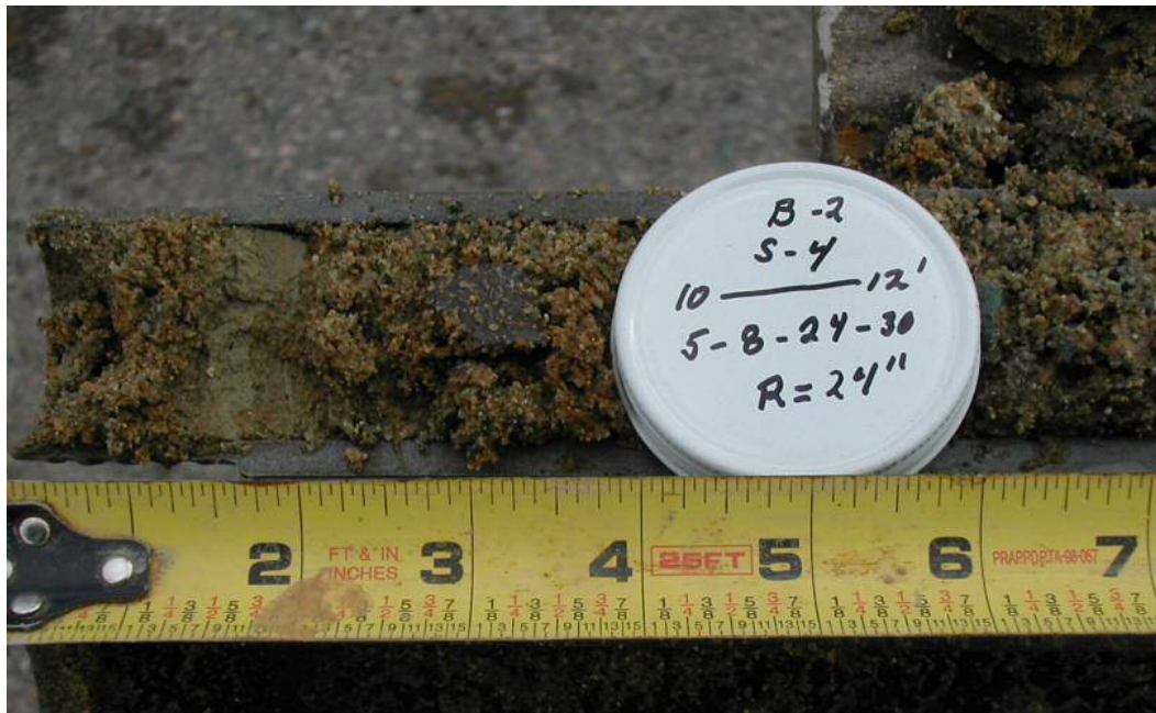
Photo 11: Test boring B-2, S-4 consisted of Gravelly Sand, stratified, mostly m-f Sand, 5-15% fine subrounded to angular Gravel, <5% nonplastic Fines, saturated, brown.
