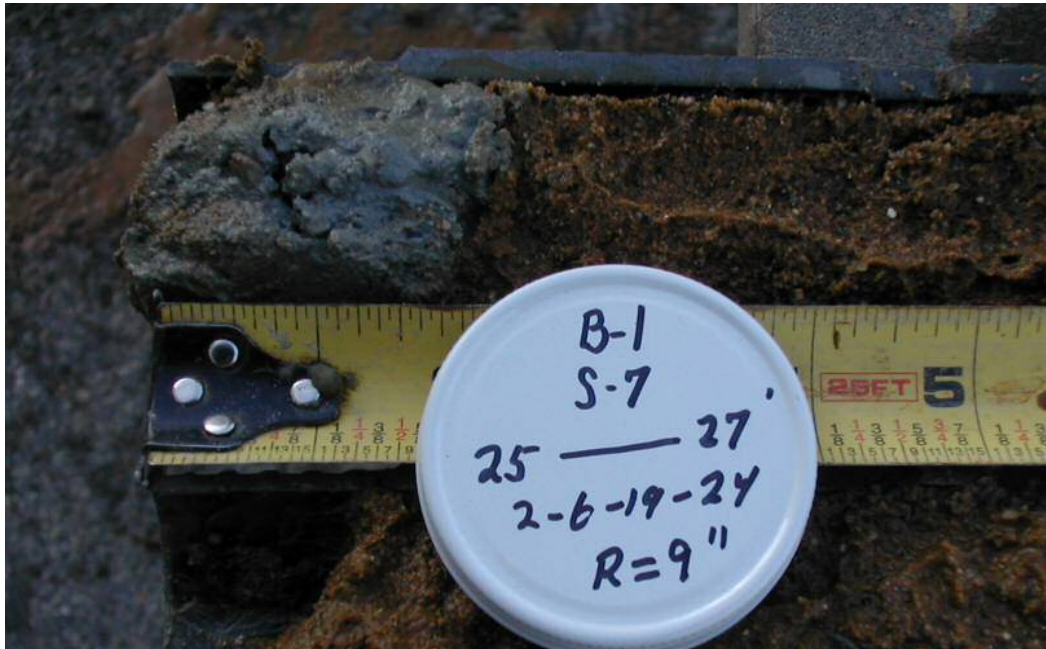
Photo 7: Test boring location B-1, S-7: Sand, mostly m-f Sand, <5% nonplastic Fines, saturated, rusty brown over Till consisting of gray Silty Gravel, m-f angular Gravel, saturated.
