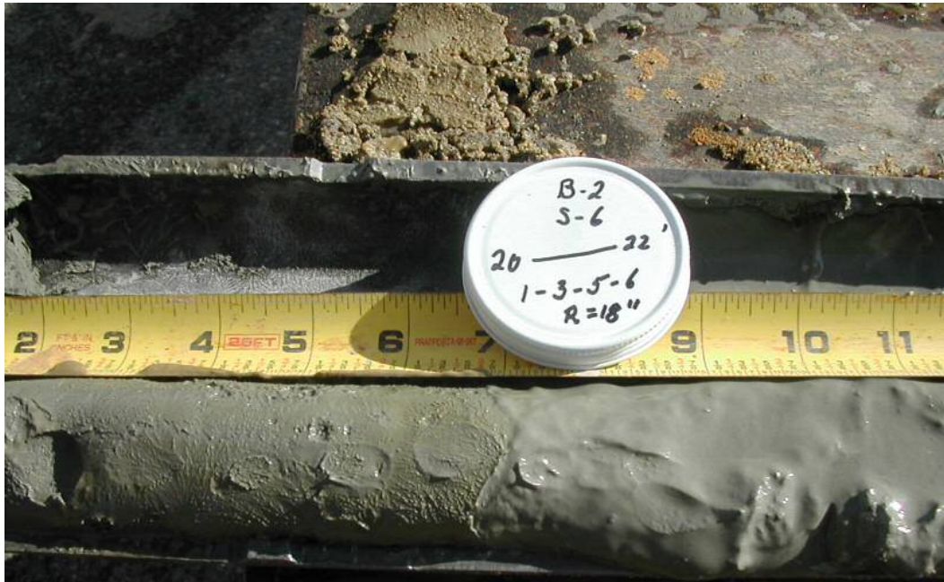
Photo 13: Test boring B-2, S-6 consisted of Clayey Silt, non- to slightly plastic Fines gray.
