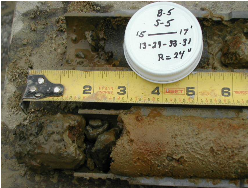
Photo 26: Test boring B-5, S-5: Till: Silty Gravelly Sand, c-f Sand, 25-35% subrounded to angular m-f Gravel, 5-15% nonplastic Fines, saturated, orange brown. Auger refusal at 18.0 ft.
