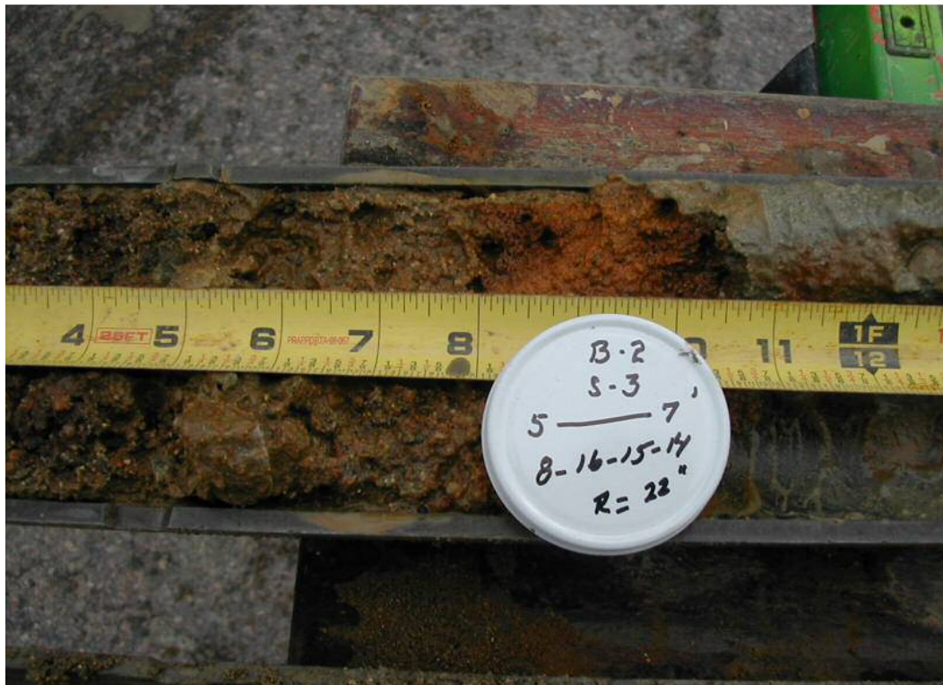
Photo 10: Test boring B-2, S-3: Silty Gravelly Sand, c-f Sand, 25-35% subrounded to angular m-f Gravel, 5-15% nonplastic Fines, saturated, brown with orange rusty brown.
