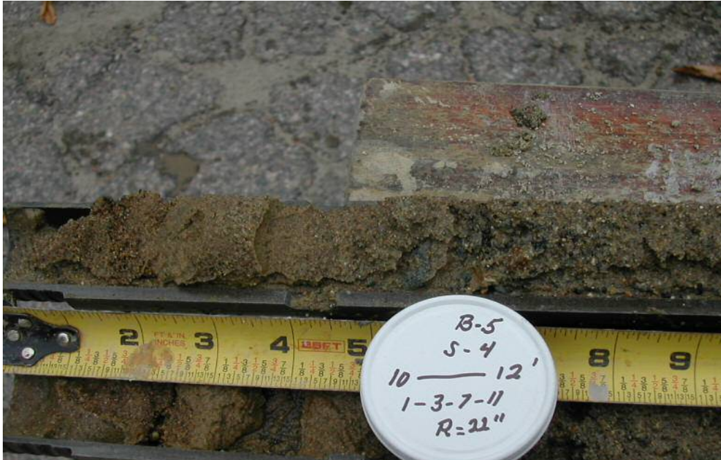
Photo 25: Test boring B-5, S-4: Sand, stratified, mostly m-f Sand, <5% m-f Gravel, <5% nonplastic Fines, saturated, brown.
